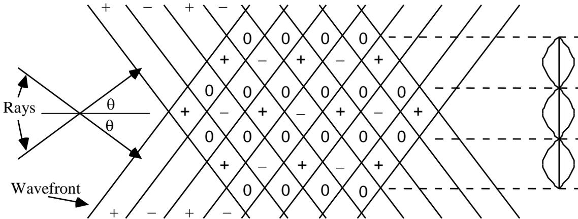
The wave fronts in the figure mark the boundaries between crests (marked +) and troughs (marked -).
