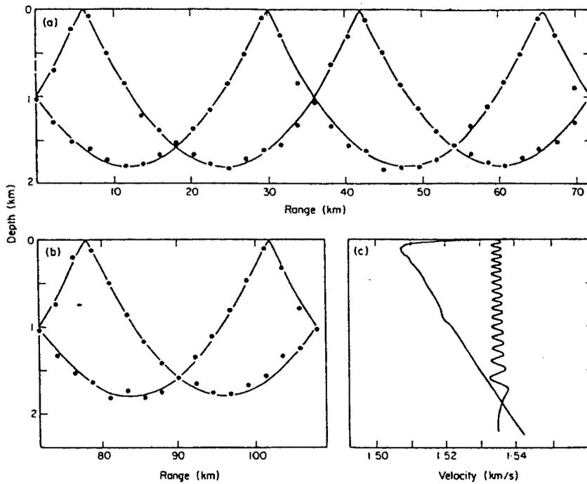
Figure (a) and (b) The dots show the depths of the peaks of the pressure envelopes as a function of range for modes 26 to 34 at 100 Hz. The solid line is a ray trace for the ray equivalent to mode 30. (c) The velocity profile [11] with mode 30 (in arbitrary units) superimposed at the correct phase velocity.
