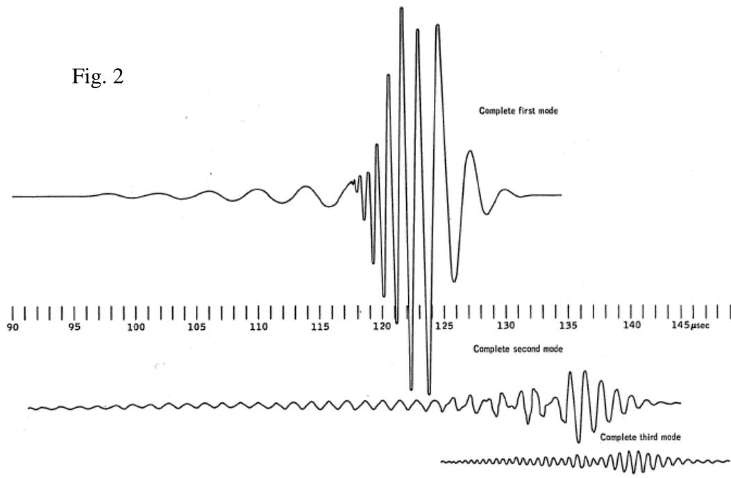
Fig. 4.14 Calculated excitation of three modes for the source of  $Q(t) = A t e^{-\lambda t} \sin \alpha t, t \geq 0$ , in the model experiment with two-layer waveguide (Sec. 4.4).
