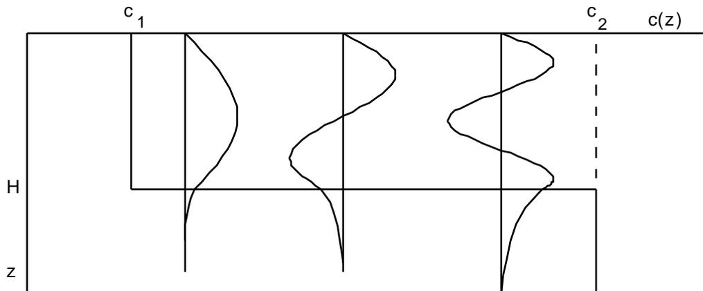
It is conventional to plot each normal mode superimposed on the velocity profile at its phase velocity  $\omega/k_n$ .
