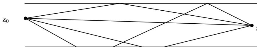
About 50 eigenrays with beam displacement contribute to the signal at the receiver.
