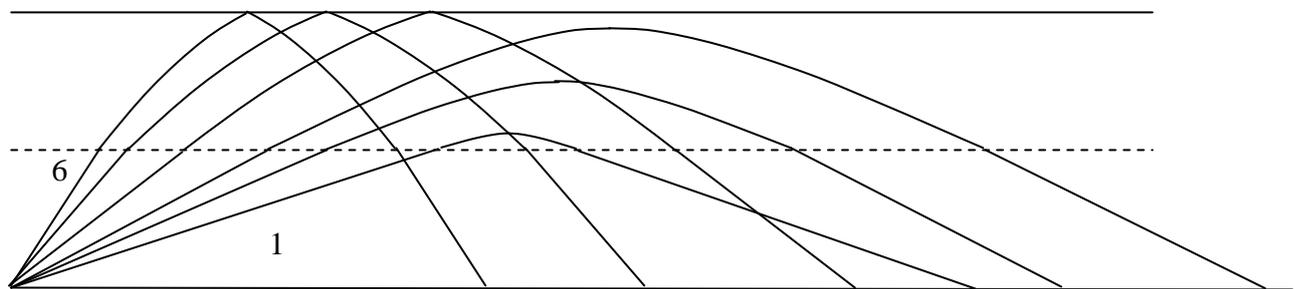
A source in the lower half will excite all modes (unless it is on a null). Mode 3 will arrive first because the equivalent ray spends longer in the higher speed layer and has the longest cycle distance. Arrival order will probably be 3, 2, 1, 4, 5, 6 i.e. order of decreasing cycle distances. A receiver near the surface will not receive modes 1-2.
