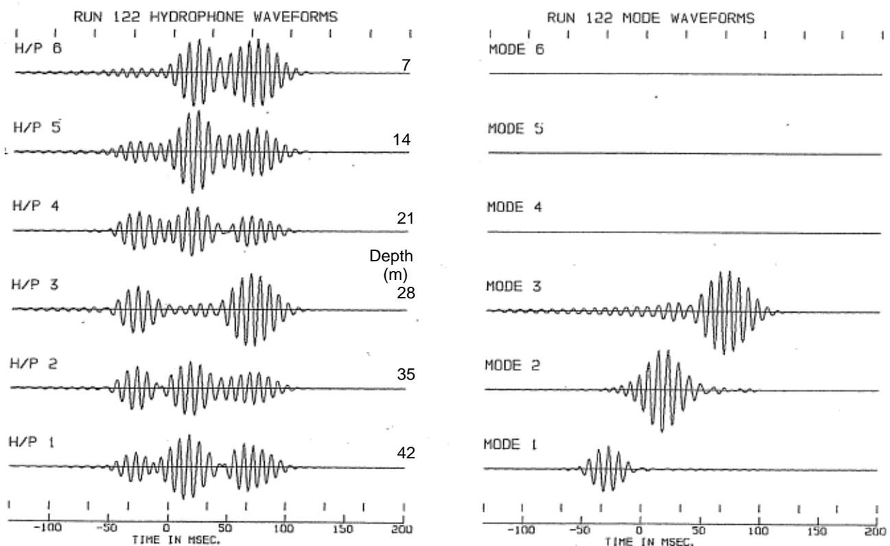
The left figure shows theoretical waveforms corresponding to the Hauraki Gulf experiments. When compared with the experimental waveforms there is excellent agreement of relative arrival times, pulse shapes and mode shapes as a function of depth. The relative mode amplitudes do not agree because attenuation was not included in the theory. The ratio of amplitudes of theory and experiment was used to measure attenuation.
