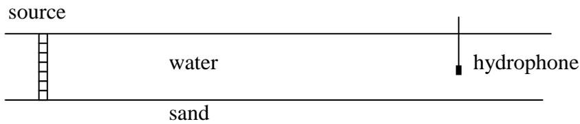
The experimental arrangement had a layer of water 10 cm deep and sound speed 1490 m/s over a sand bottom of sound speed 1784 m/s. The density ratio was 1.97.
