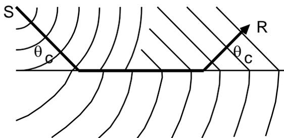
This arrival is usually called the head wave in seismology. It travels down to the boundary at the critical angle, along the interface at the speed of the lower medium and up to the receiver at the critical angle. The waves in the lower medium continually radiate up into the upper medium.
