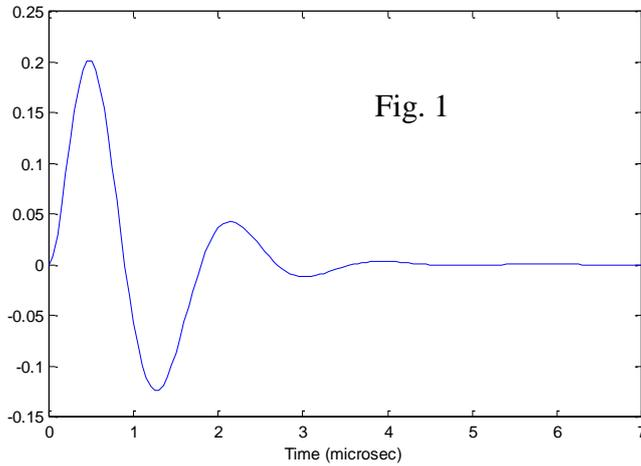
The source pulse is effectively a one cycle pulse at 560 kHz. It has a wide bandwidth with most of the energy in the 280 - 840 kHz band.
