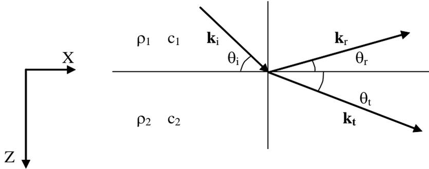
Assume an incident plane wave produces a reflected plane wave and a transmitted plane wave. Wave number vectors  $\mathbf{k}_i$ ,  $\mathbf{k}_r$  and  $\mathbf{k}_t$  as shown. Note that we have not assumed  $\theta_r = \theta_i$ .
