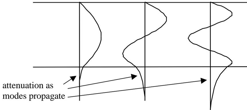
Mode amplitude decays with range as the bottom absorbs energy. Usually higher modes decay more rapidly.
