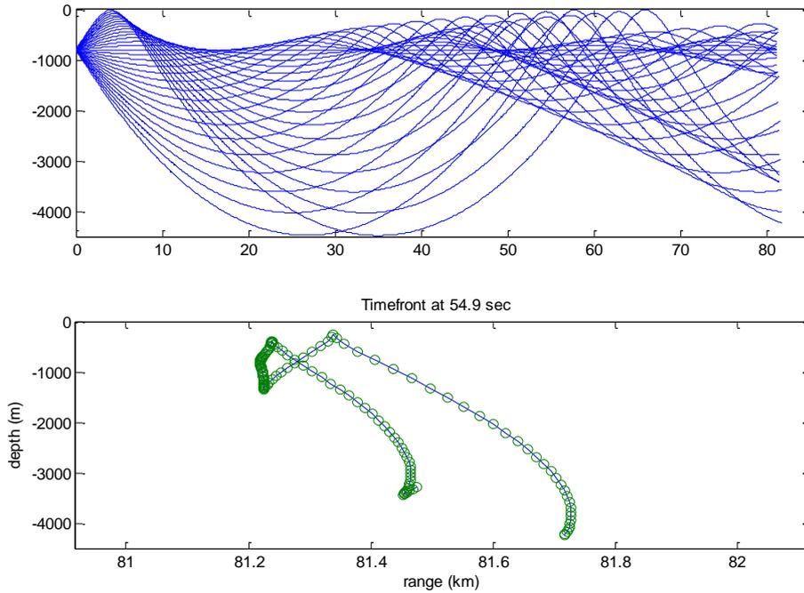
If the wavefront passes a vertical array the time order is reversed as in the left diagram below.
