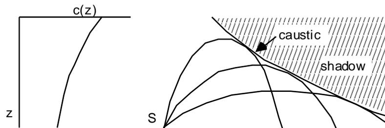
A caustic is formed when a series of rays of slightly different angles form a boundary between a shadow zone where the rays do not reach and an insonified zone where there are two rays through each point. Each ray touches the caustic in a different place. Simple ray formulas must be modified near focusses and caustics to avoid prediction of infinite energy.
