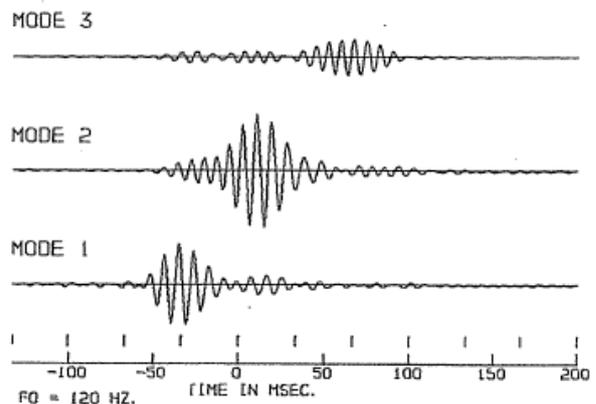
The source transmitted a smoothed four cycle cosine pulse at 120 Hz as shown.
