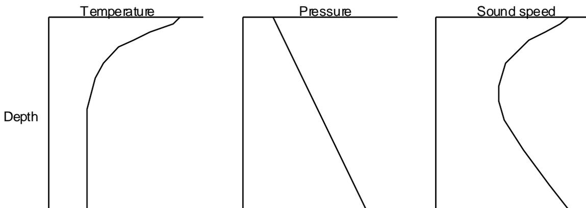
Sound speed at the ocean surface is  $1508 \text{ m/s}$  for a temperature of  $15^\circ\text{C}$ .
