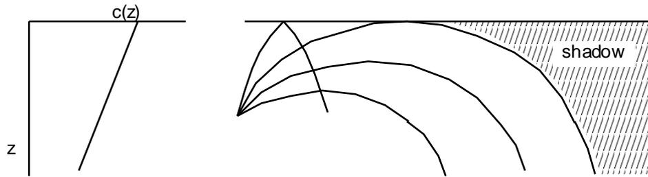
A shadow zone is a region where sound cannot reach along a ray path. In the situation shown the ray which grazes the surface forms a boundary between the insonified region and the acoustic shadow. Sharp shadows are impossible. There is always diffraction into the shadow region and ray theory must be modified to find the field in shadows.
