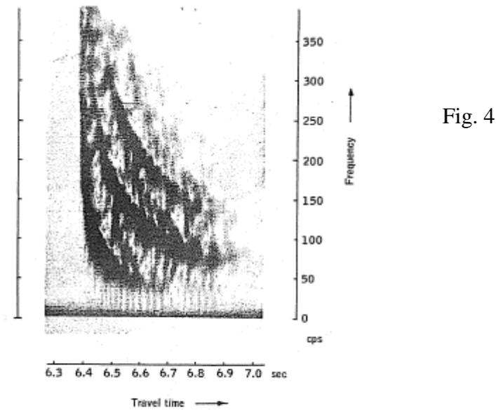
Fig. 4.10 Group-velocity curves displayed by a spectrum analyzer for typical shallow-water shot: 12 kg of TNT at 9.7 km distance in 30 m of water. (Courtesy of J. B. Hershey, Woods Hole Oceanographic Institution.)
