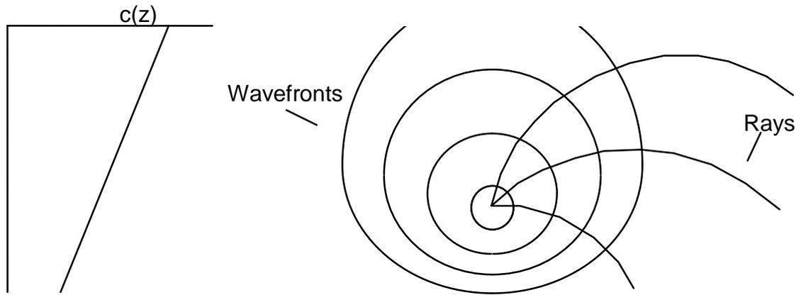
Rays curve towards the minimum of sound speed. In deep water they cycle up and down about the sound speed minimum.
