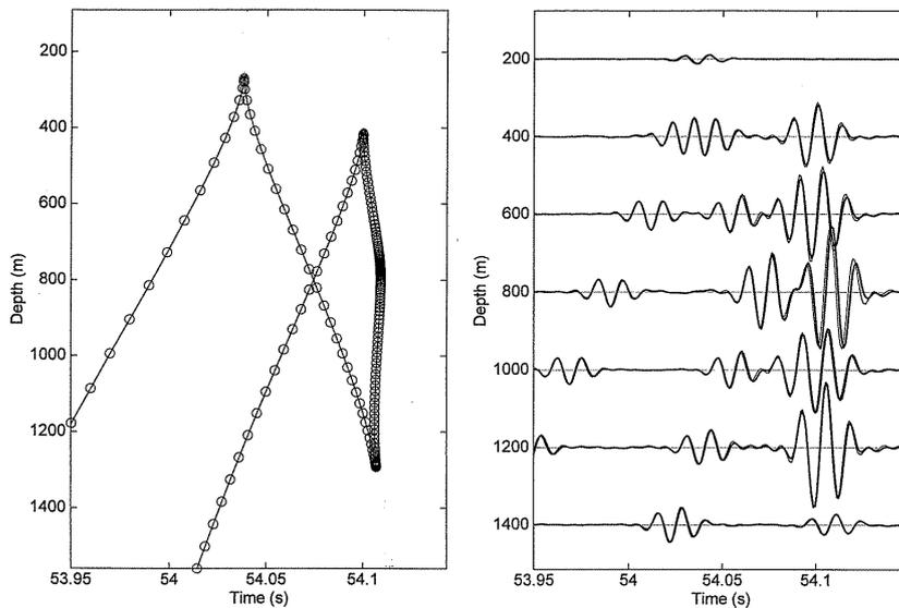
The right figure above shows the waveforms that would be measured if the source emitted a two cycle pulse at 75 Hz. The modelled waveforms include pulses in the geometric shadow. [Tindle JASA 112, 464-475 (2002)]
