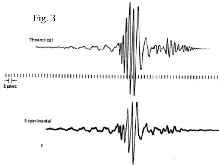
Fig. 4.15 Superposition of the three calculated modes of Fig. 4.14 (theoretical curve) compared with experiment for the two-layer waveguide model.
