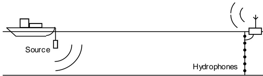
In a shallow water normal mode experiment a sound source transmits to a vertical array of hydrophones. The received signals are transmitted back to the ship and recorded.
