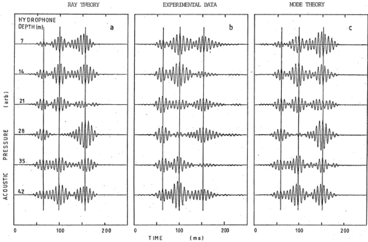
The waveforms on all six hydrophones are shown in the figure.
