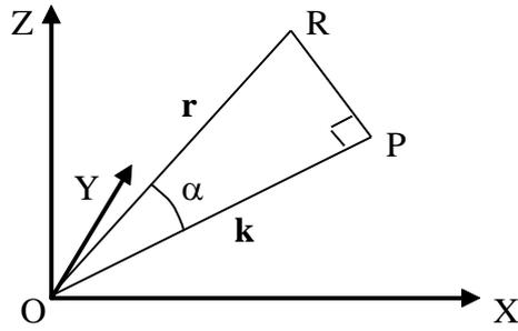
Let R be an arbitrary point on the wavefront through P.  $RP$  is perpendicular to  $OP$ .
