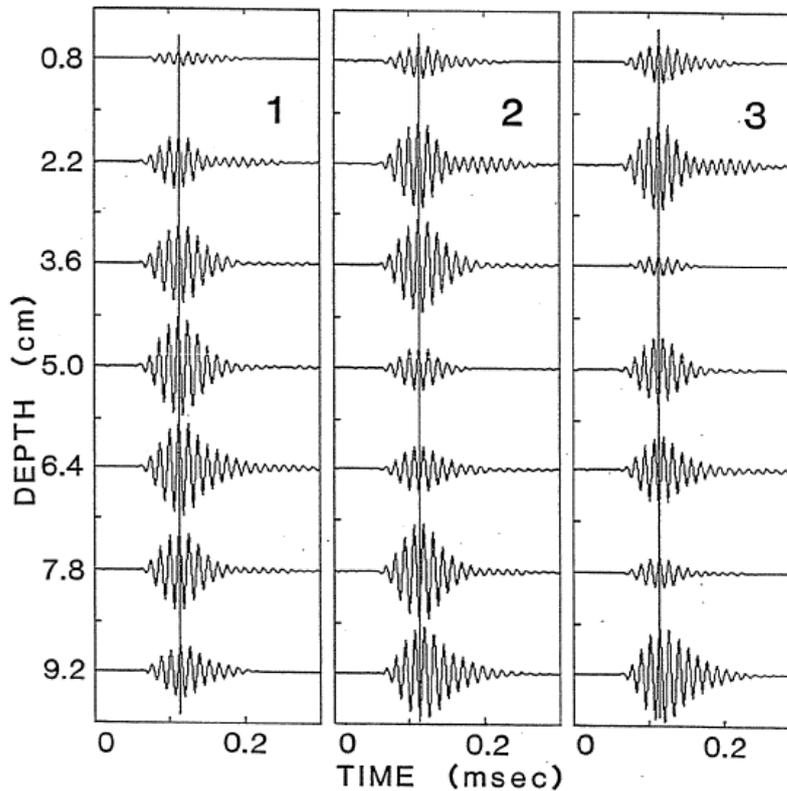
Figure 1 shows the source waveforms at the source element depths for the first three modes. The vertical lines and the peaks in the waveforms show that for mode 1 all sources are in phase. For mode 2 the upper four sources are in phase and the lower three are phase reversed. For mode three the upper three sources are in phase, the next two are phase reversed and the lower two are in phase with the upper three.
