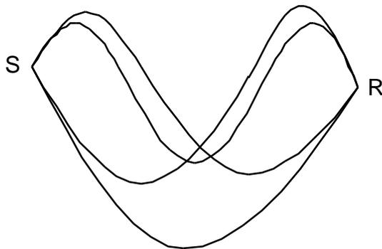
The four eigenrays with one lower turning point.
