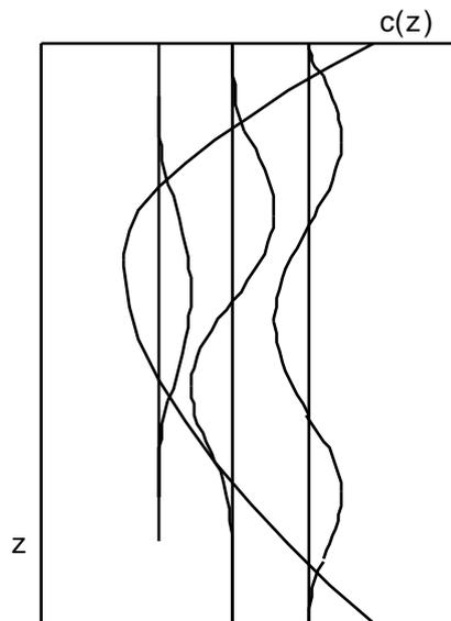
The eigenvalues for these modes are not determined by the boundary conditions. Instead they are determined because the exponential and oscillatory solutions must match smoothly at the turning points. Smooth matching means that both value and derivative must be continuous. For an arbitrary value of  $k$  the solutions will usually not match. The value of  $k$  is adjusted until a match occurs.
