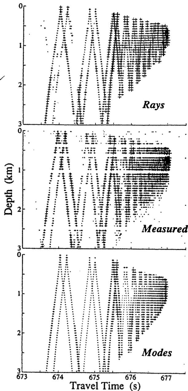
The middle panel is data. The top and bottom panels are modelled using rays and modes respectively in the average sound speed profile.
