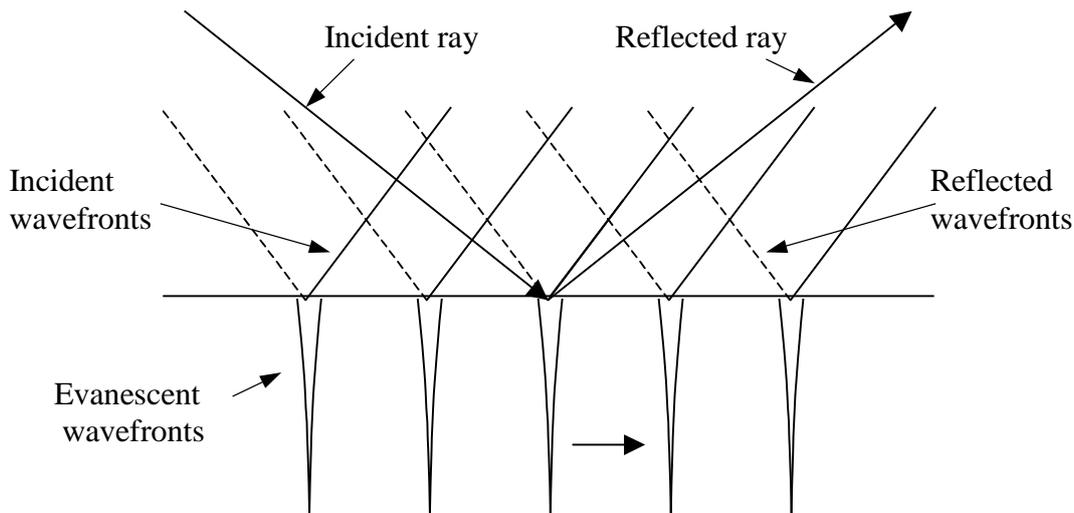
The field in medium 2 travels parallel to the boundary with wavefronts perpendicular to the boundary. There is exponential decay of amplitude away from the boundary. Such waves are called **evanescent waves** or **inhomogeneous waves** and satisfy the wave equation.
